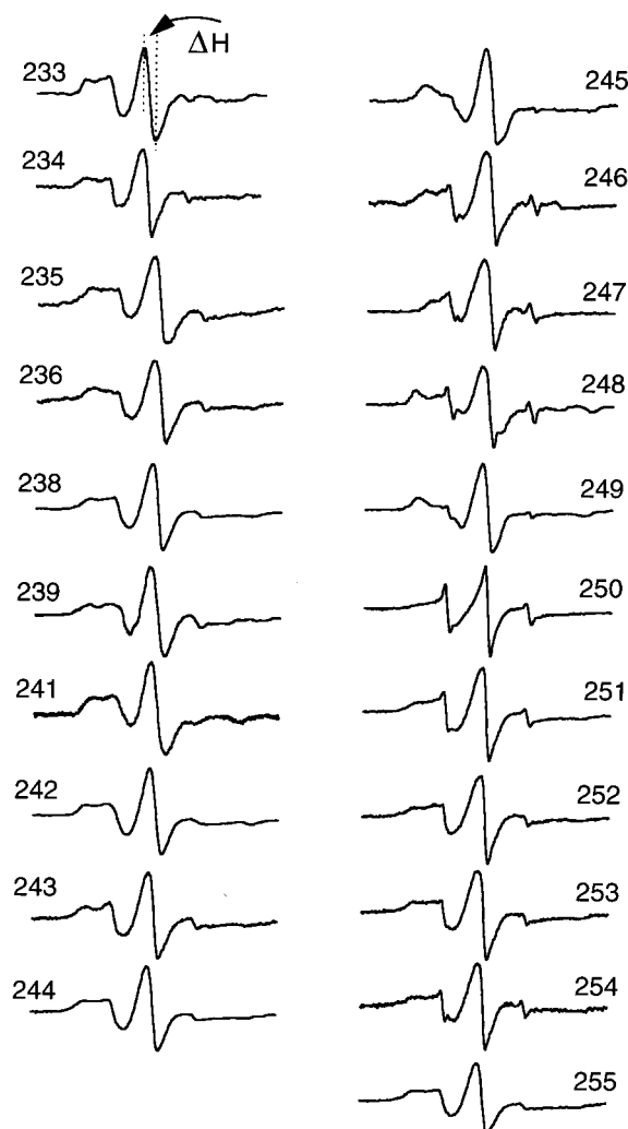
FIGURE 3: First-derivative EPR spectra of given nitroxide-labeled single-Cys mutants at positions 233–255, excluding positions 237 and 240 which were examined previously (16). The spectra are scaled vertically for convenience of presentation, and the magnetic field scan width is 98 G. The line width of the central resonance ( \Delta H ) is indicated on the spectrum of residue 233.
